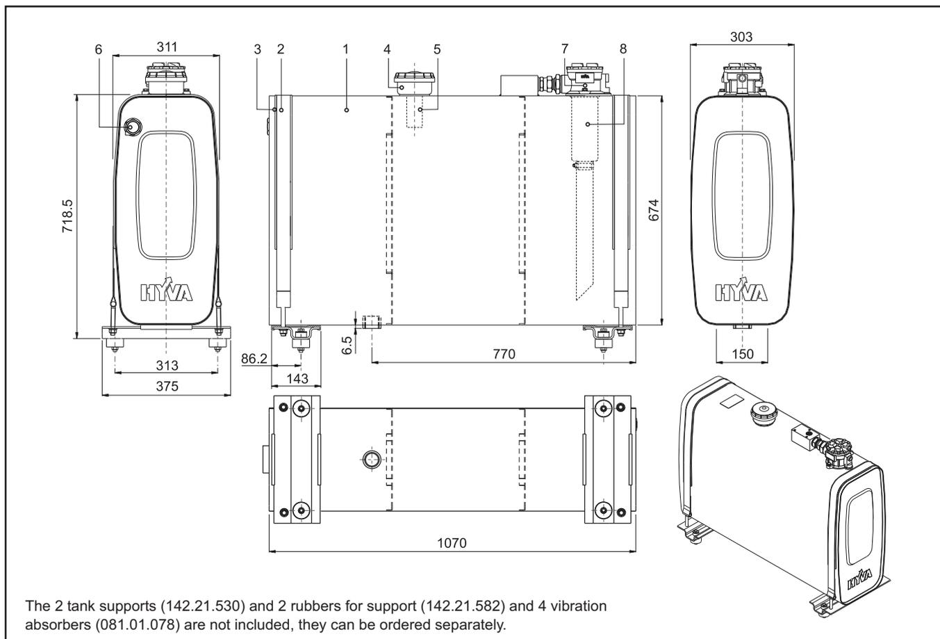
The 2 tank supports (142.21.530) and 2 rubbers for support (142.21.582) and 4 vibration absorbers (081.01.078) are not included, they can be ordered separately.
